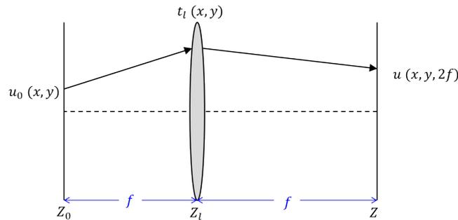
Figure 2: Geometry for optical propagation through a lens.
