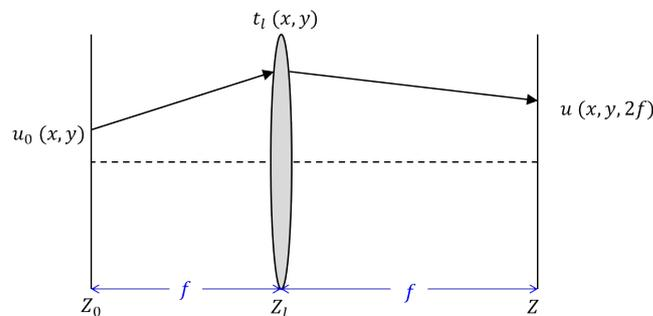
Figure 1: Geometry for optical propagation through a lens.
